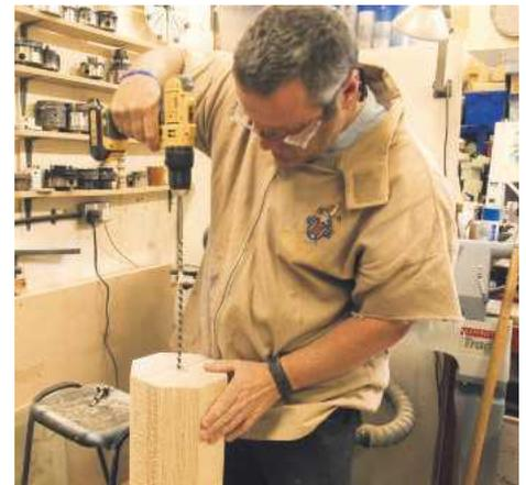
▲ Pic.6 Use the drill press to part drill a 7mm hole in from each end and then complete the through hole with a beam drill. For greater accuracy use the usual long-hole boring method
